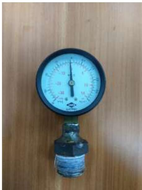
**Gambar 14.** *Pressure Gauge (Section)*
